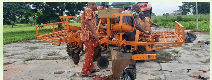
The planter is being repaired for the broken parts after the second day of work. This took 3 days to complete
